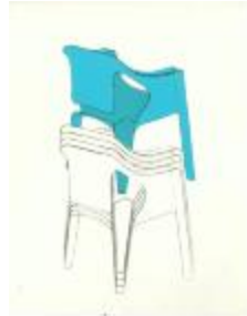
Reproduction of drawing depicting how chairs can be stacked (KA0123_kOSx4_f10_04)
